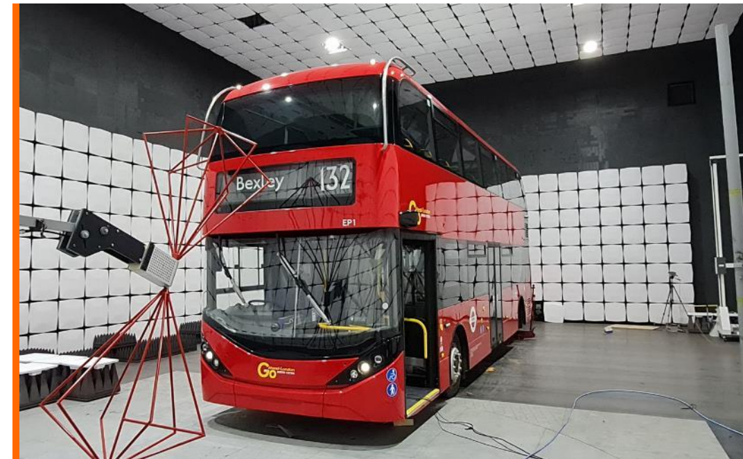
An electrified British double-decker bus tested in our full-vehicle EMC chamber in the UK.
